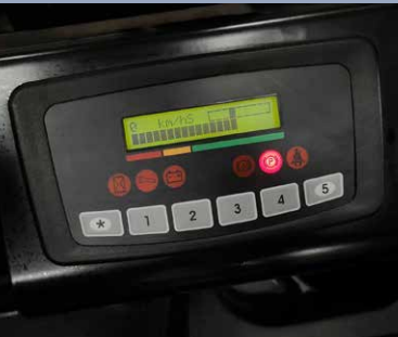
Steering angle display can help improving safety during driving
